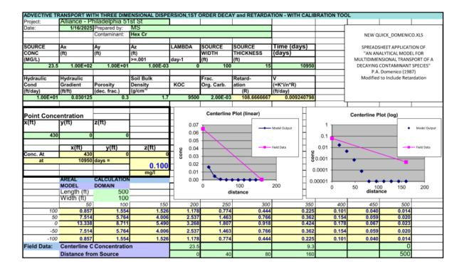
The data shows a source concentration of 23.5 mg/L at MW-4, and a predicted centered concentration of 13.3 mg/L 50 feet east of MW-4. From this point, the plume spreads:
