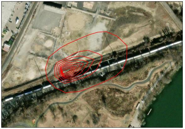
The above plume graphic with labeled isolines (contour lines) showing the predicted Chromium VI concentrations in mg/L. The white line marks the 0.1 mg/L PADEP threshold, while the black isolines provide a clear view of predicted concentration gradients across the site.
